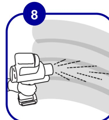
**8** When applying the solution with this technology, make sure you move at an even pace to ensure the surfaces are thoroughly covered. Apply solution using a slow sweeping motion across the surfaces and allow the spray to overlap when moving to the next section. Follow a continuous path through the room at a smooth pace, moving backward toward the door, spraying away from your body and not walking into the spray.
