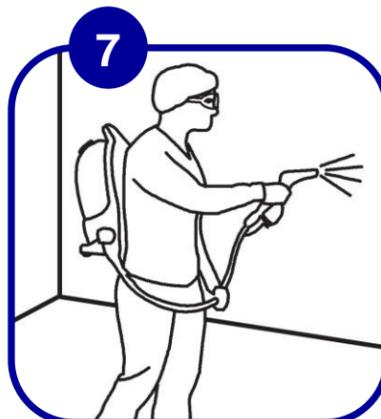
**7** Review the manufacturer instructions in the sprayer device manual and follow accordingly. Position in a rear corner of the area to be sprayed. Direct the sprayer to the desired surface area and begin to spray. Review the disinfectant label, and ensure you understand the contact time necessary for the surface to remain wet for efficacy.
